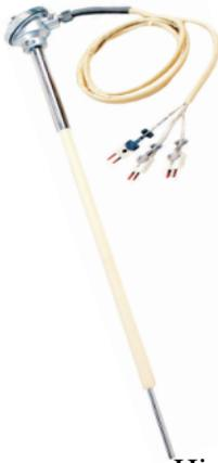
Thimbles made of special platinum alloy containing 10% Rhodium with small% of Zirconium oxide or yttrium oxide (as grain stabilizer), are developed specially for the application in glass industries.
